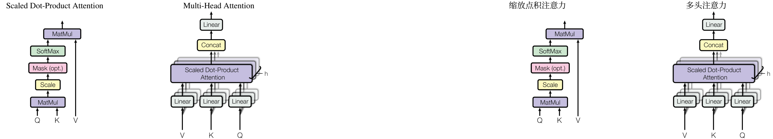
Figure 2: (left) Scaled Dot-Product Attention. (right) Multi-Head Attention consists of several attention layers running in parallel.
